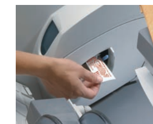
Auto Tape Mode sets the system to generate a tape when heavier material is placed on the scale.
